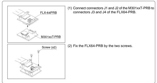
Figure 3.9 Connecting pod probe M301xxT-PRB
